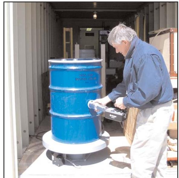
Fig. 9. Scanning for a "Hot Spot."
