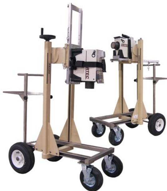
Fig. 3. ISO-CART with trans-SPEC-100.
