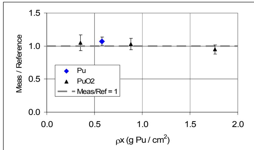
standards (0.579, 0.881 and 1.762 g Pu/cm<sup>2</sup>) are, respectively, two, three and six times thicker than the upper end of the thickness range for expected holdup deposits. The corresponding self-attenuation corrections are approximately 9%, 12% and 22%. Ignoring the correction causes a negative bias in the measurement result in all cases. Corrections for self-attenuation effects have not been included in analysis procedures for holdup measurements traditionally.
