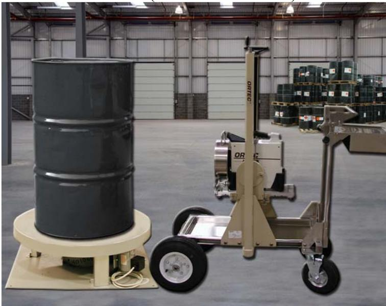
**Figure 1. A measurement station using a trans-SPEC.**
