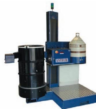
Gamma-ray peak areas from the sample emission spectrum are used to determine the activity of radionuclides in the segment. The peak areas are corrected for attenuation using the data obtained during the transmission measurement. Alternatively, if no transmission source is used, the activity is determined by comparing the peak areas to the equivalent peak areas obtained from calibration measurements for an assumed equivalent matrix.
