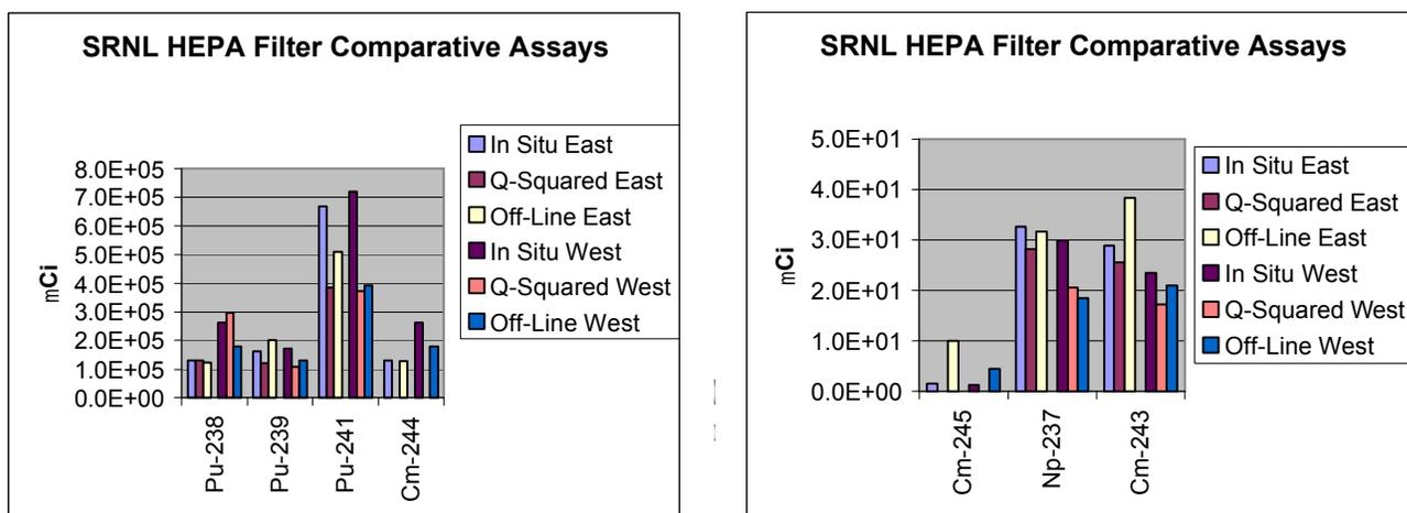
**Figure 5. Comparison of measured contents (or MDA's) between the final in-situ assays, the Q<sup>2</sup> assays, and the off-line assays for the SRNL East and West glovebox HEPA filters.**
