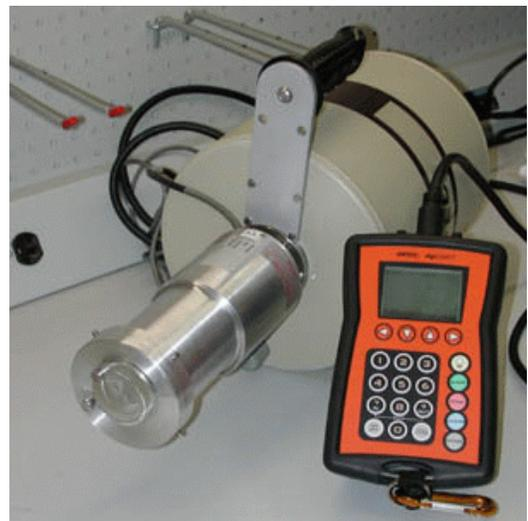
**Figure 2** The portable MCA in hand-held use
