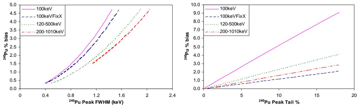
**Figure 2. Pu-240 biases as the functions of the FWHMs and of the tails of the  $^{240}\text{Pu}$  peaks. The  $^{240}\text{Pu}$  peak is the 104.2-keV peak for the 100-keV region analysis, 160.3-keV peak for the 120- to 500-keV region analysis, and 642.5-keV peak for the 200- to 1,010-keV region analysis.**
