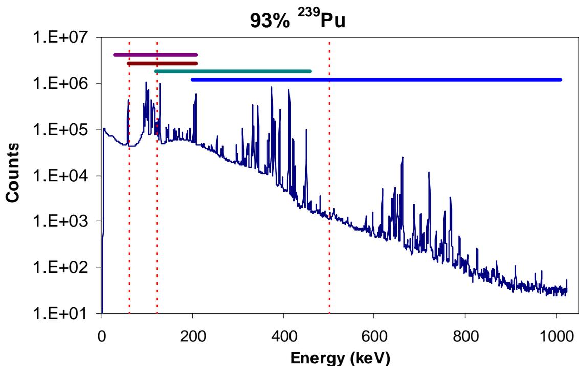
**Figure 1. A low-burnup plutonium spectrum. The three vertical, dashed lines separate the four regions. The four overlapping analytical regions that FRAM normally uses for the analysis are shown as four thick horizontal bars above the spectrum.**
