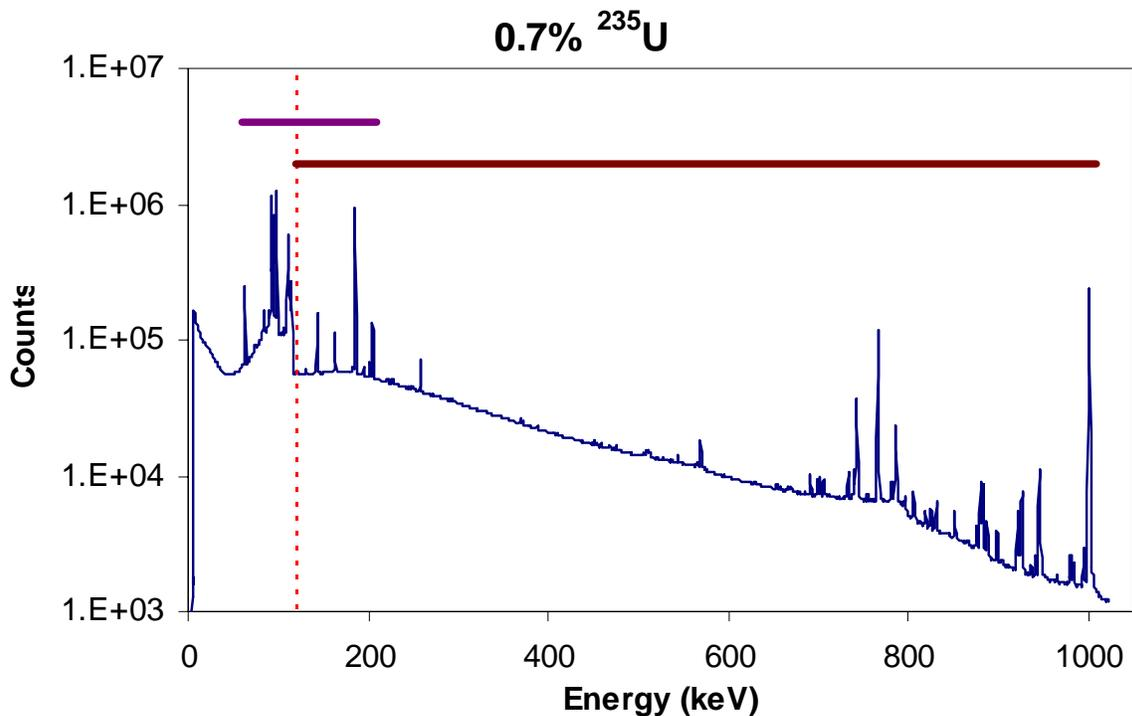
**Figure 3.** A natural-uranium spectrum. The vertical dash line separates the two regions: one below the K-edge and one above the K-edge. The two overlapping analytical regions that FRAM normally uses for the analysis are shown as two thick horizontal bars above the spectrum.
