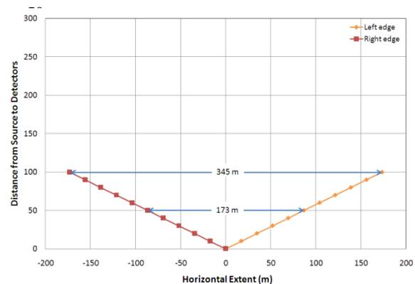
Figure 5 Width of 120° FOV at various distances
