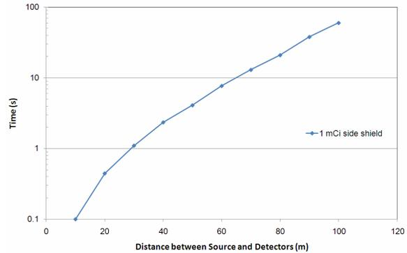
Figure 13 Time to Detect by Distance for 8 IDMs
