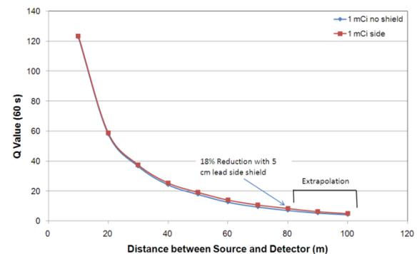
Figure 12 Q Based on 8 IDMs for Different Shielding
