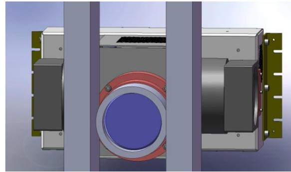
Figure 3 IDM with side and cylindrical shielding
