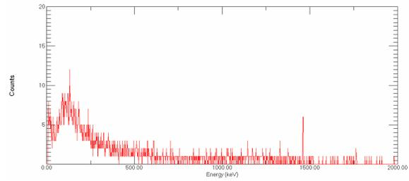
Figure 6 Background with no Extra Shielding (60 s)
