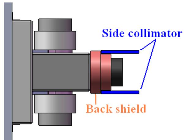
Figure 3. IDM with Shielding to Limit Background
