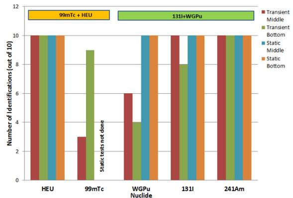
**Figure 11. Nuclide Mixture Identification in Unshielded Mode**
