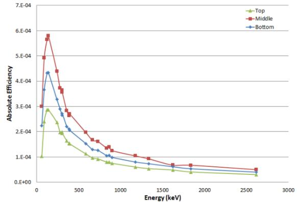
**Figure 3. Efficiency vs Energy for the Source at Three Different Heights and Horizontally Centered.**
