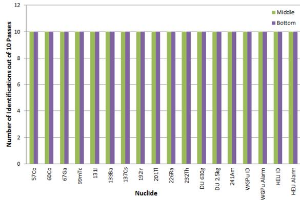
**Figure 7. Single Nuclide Identification in Static Mode (Unshielded)**
