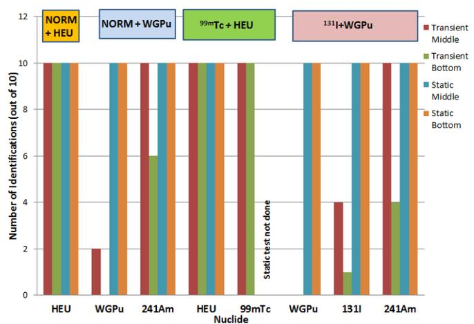
**Figure 12. Nuclide Masking Identification in Unshielded Mode**
