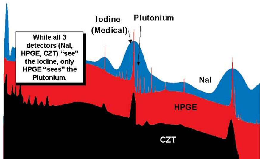
Figure 2. HPGe in comparison to NaI and CZT detectors.
