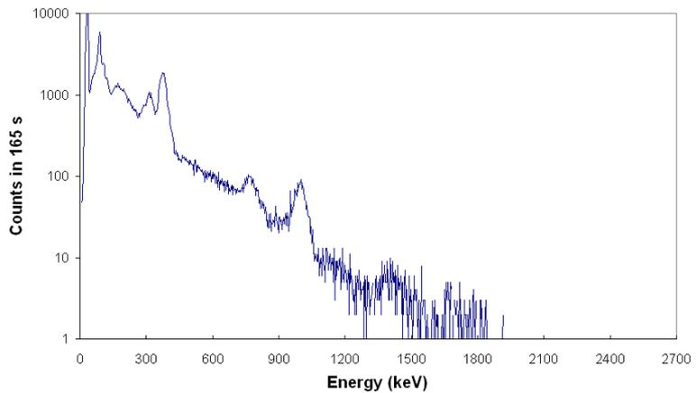
Figure 5. Scintillator spectrum of depleted uranium and <sup>133</sup>Ba.
