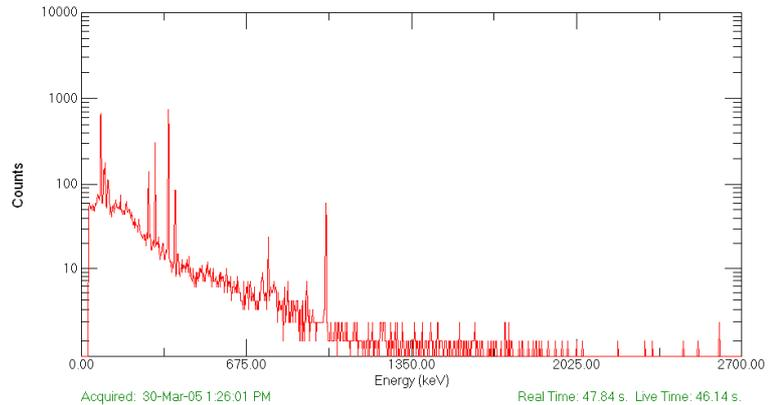
**Figure 3.** HPGe Spectrum of depleted uranium and  $^{133}\text{Ba}$ .
