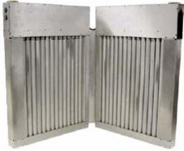
**Figure 3** Instrument hardware showing 3He tubes
