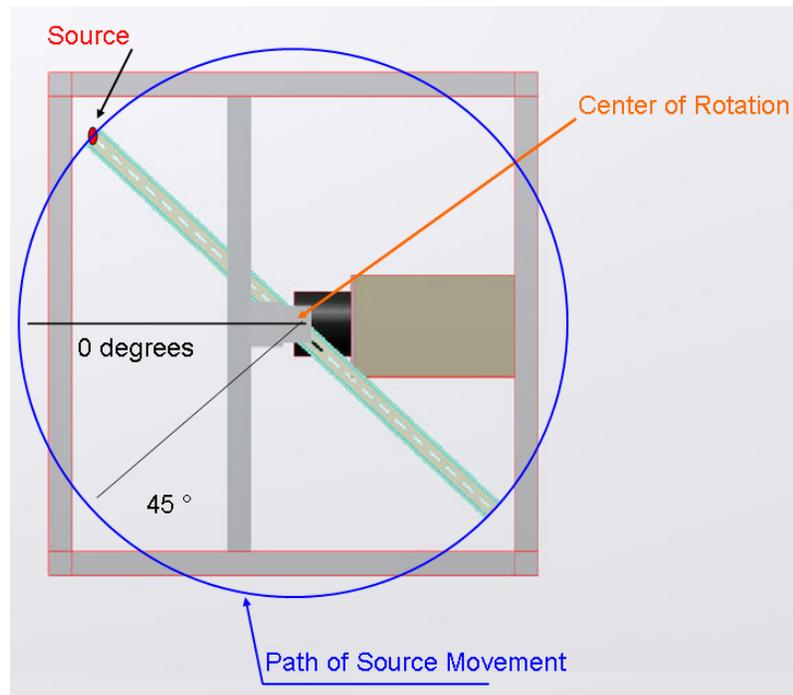
**Figure 4 Angle Definition for Source Position Around Detective 100**
