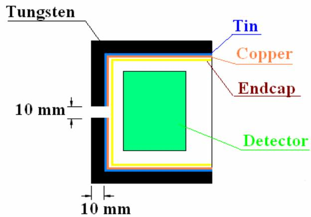
Figure 2 Collimator Construction
