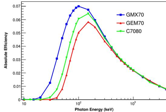
Fig. 6. Calculated efficiency versus photon energy for an aqueous source in a Marinelli beaker.
