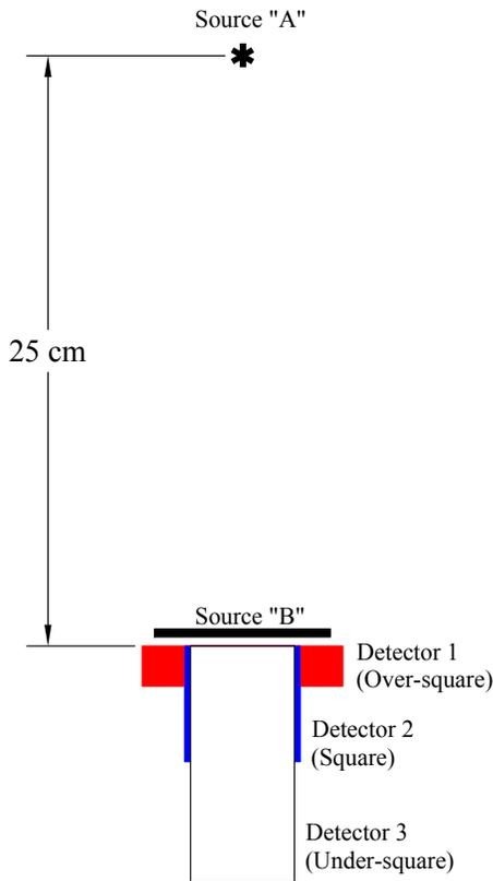
Fig. 3. Schematic representation of three detectors with the same IEEE relative efficiency (source "A" at 1332 keV), but widely different absolute efficiencies with respect to low-energy source "B".
