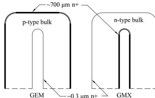
Fig. 2. Conventional HPGe detector configurations.
