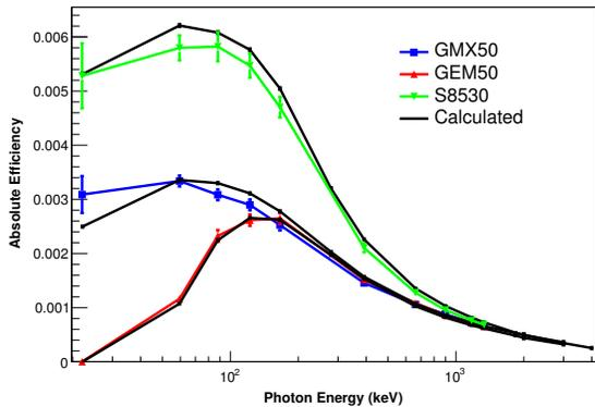
Fig. 4. Measured and calculated efficiency versus photon energy for a point source at 25 cm.
