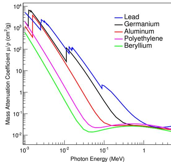
Fig. 1. Mass attenuation coefficients for a variety of materials[1].
