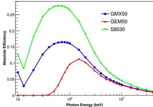
Fig. 5. Calculated efficiency versus photon energy for a filter paper source on endcap.
