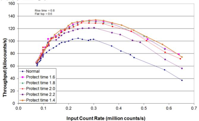
**Figure 8 Throughput for different protection times as a function of dead time with Rise Time = 0.8 and Flat top = 0.6  $\mu\text{s}$ .**
