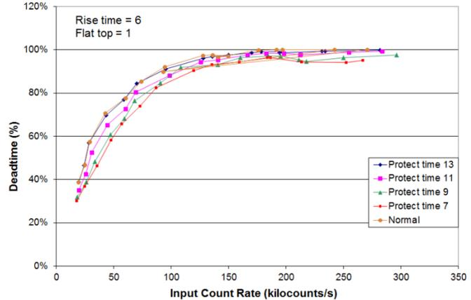
**Figure 12 Dead time vs input count rate for various protection times**
