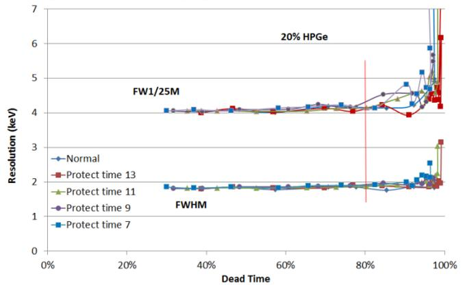
**Figure 11 Resolution vs dead time for various protection times**
