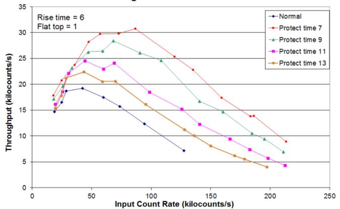
**Figure 10 Throughput vs ICR**
