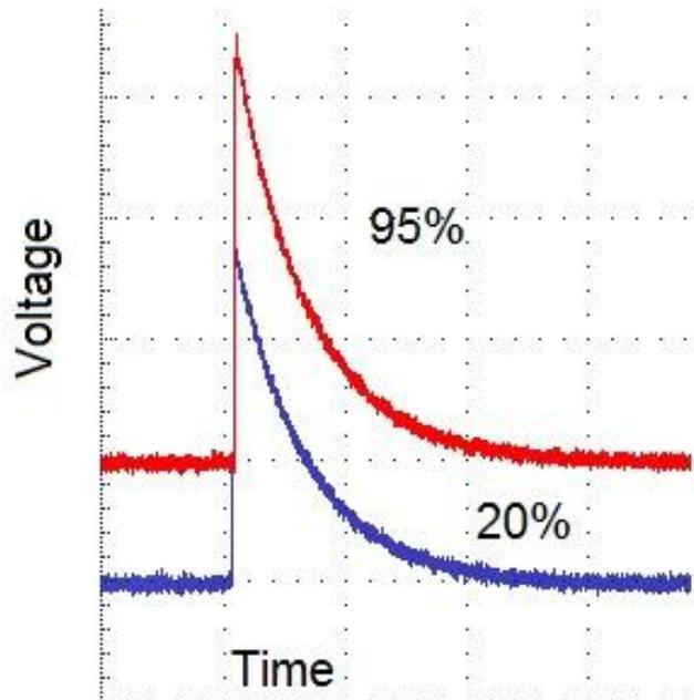
**Figure 2 Preamplifier pulses from 20% and 95% HPGe**
