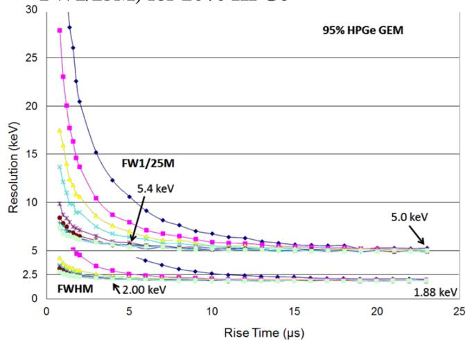
**Figure 6 Resolution at 1.33 MeV vs rise time for many flat top times (FWHM and FW1/25M) for 95% HPGe**
