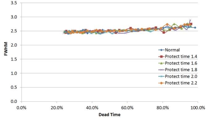
**Figure 9 Resolution at 1.33 MeV for different dead times and protection times**
