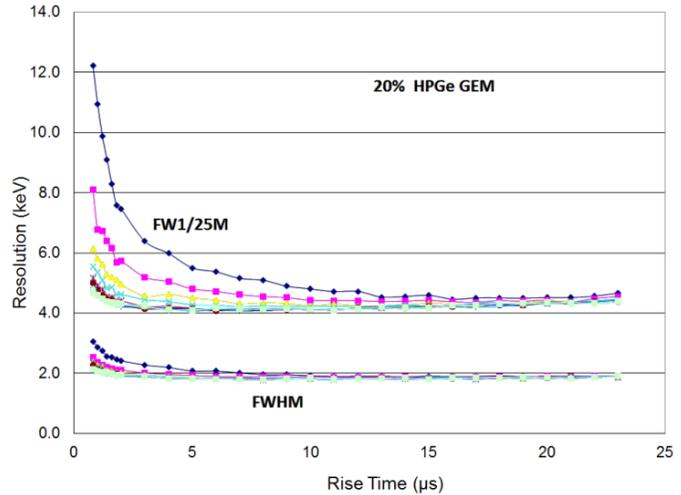
**Figure 7 Resolution at 1.33 MeV vs rise time for many flat top times (FWHM and FW1/25M) for 20% HPGe**
