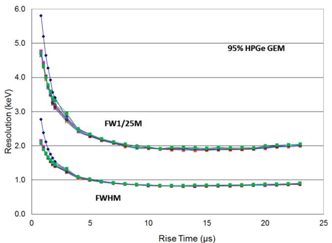
**Figure 5 Resolution at 88 keV vs rise time for many flat top times (FWHM and FW1/25M) for 95% HPGe**
