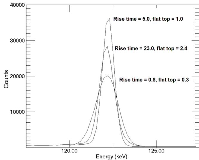
**Figure 3 Comparison of spectrum peak shapes for different shaping times**
