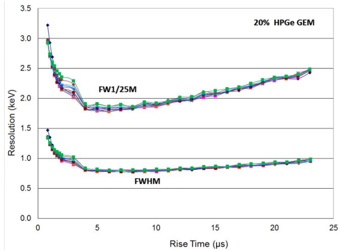
**Figure 4 Resolution at 122 keV vs rise time for many flat top times (FWHM and FW1/25M) for 20% HPGe**
