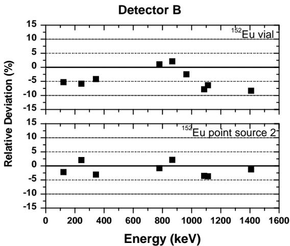
Fig. 2. Results obtained with detector B. Relative deviations between the ANGLE calculated and the experimental efficiency calibration values for <sup>152</sup>Eu point source 2 and <sup>152</sup>Eu vial standards.
