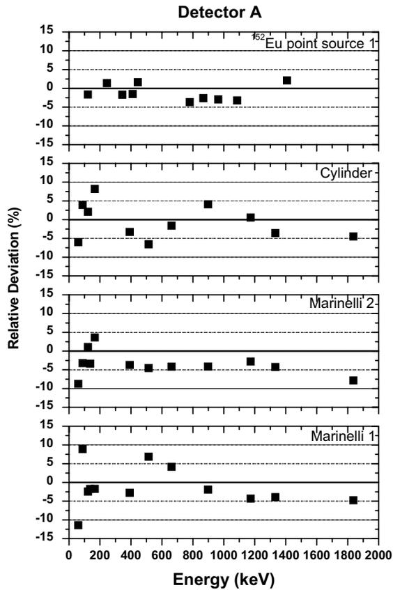
Fig. 1. Results obtained with detector A. Relative deviations between the ANGLE calculated and the experimental efficiency calibration values for <sup>152</sup>Eu point source 1, Marinelli 1, Marinelli 2 and Cylinder standards.
