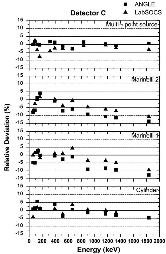
Fig. 3. Results obtained with detector C. Relative deviations between both the ANGLE and the LabSOCS calculated and the experimental efficiency calibration values for Multi- $\gamma$  point source, Cylinder, Marinelli 1 and Marinelli 2 standards.
