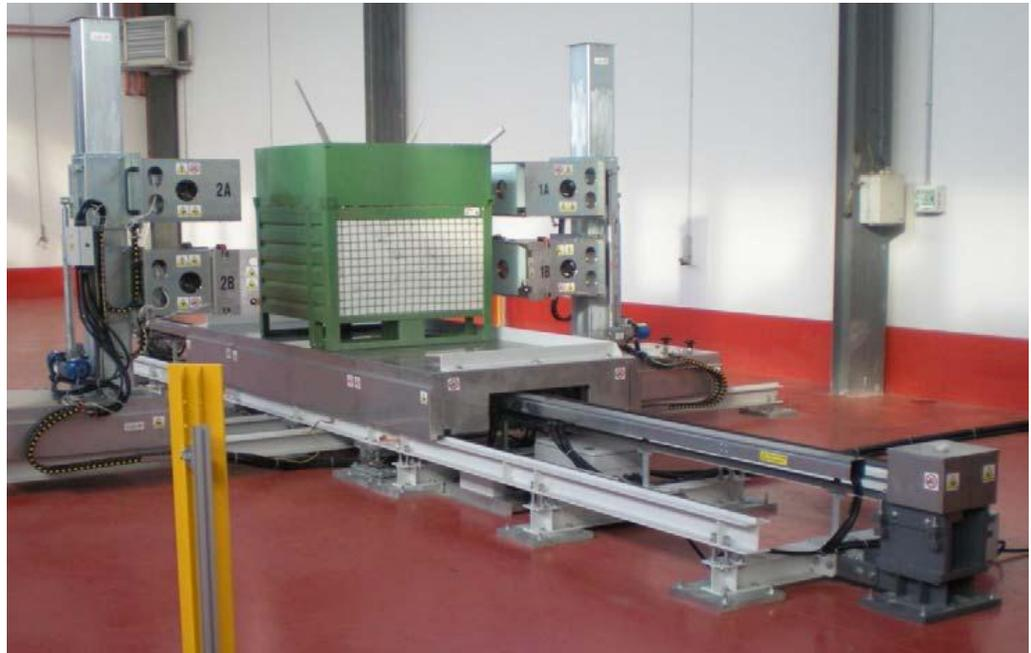
Figure 1 Example system with HPGe detectors.
