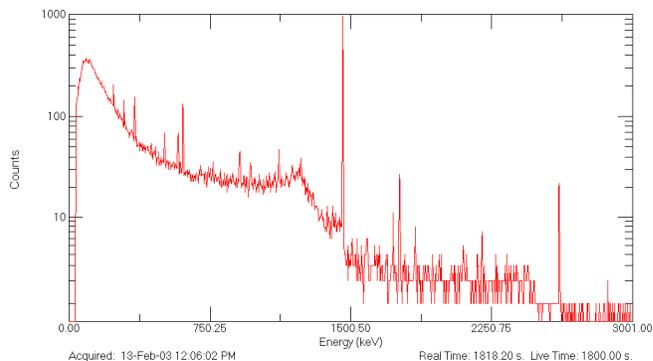
**Figure 4.** Typical Spectrum of Unshielded Potassium Chloride.
