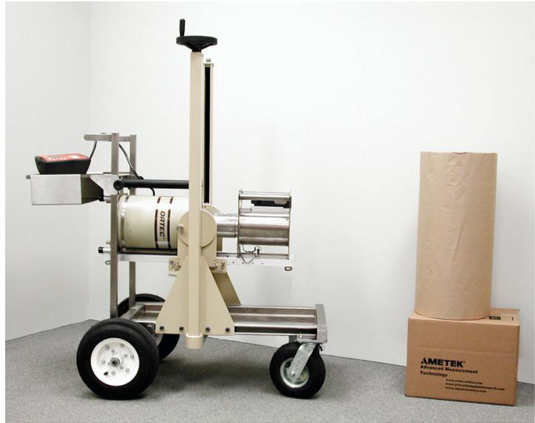
Figure 1. The ISO-Cart system for drum scanning.
