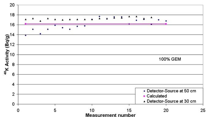
**Figure 6.** Replicate Measurements for the Same Standoff.
