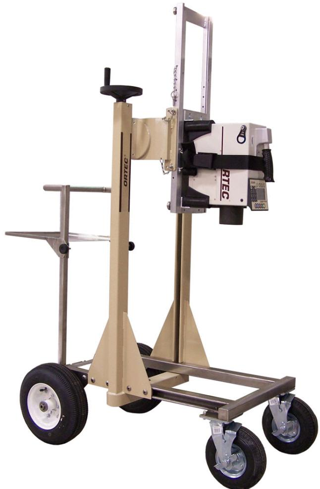
**Figure 1** Trans-SPEC-100 on Iso-Cart.
