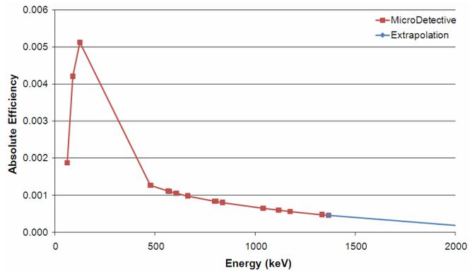
**Figure 3. Absolute Efficiency for 10 cm Disk at 10 cm**
