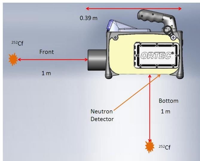
**Figure 7. Neutron Source Placement for Sensitivity Measurement**
