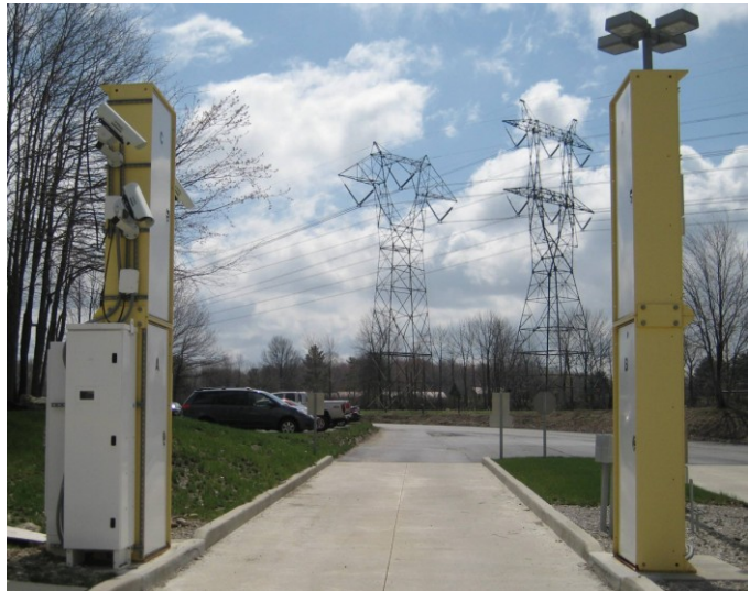
Figure 4. Typical installation of ARIS-1024 portal monitor.
