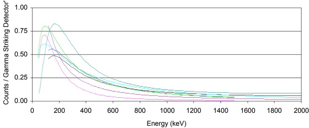
Fig. 1. Intrinsic efficiency curves for all of the instruments used in this study.
