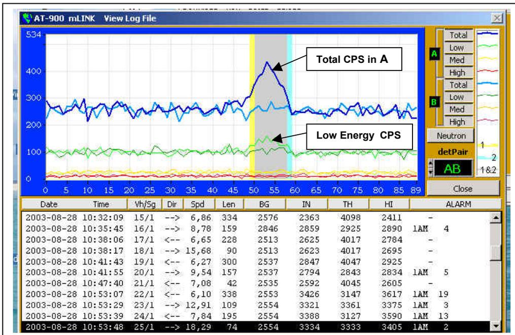
Fig. 6: Count rate profiles in three different energy ranges with a WG Pu source passing through.
