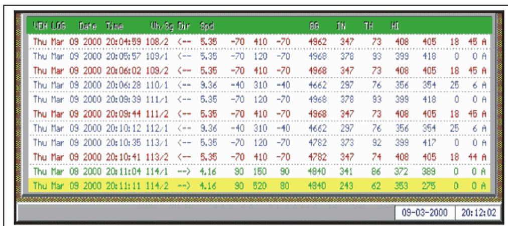
Fig.4: Display of vehicle log with time/date, speed, count rate and threshold data
