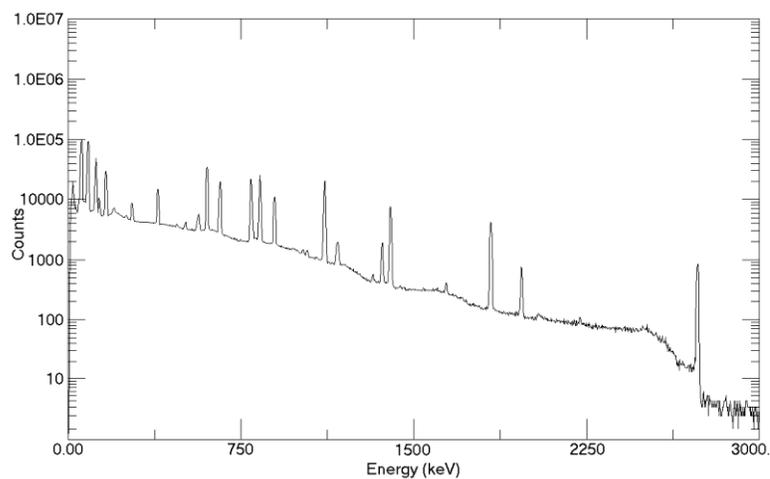
**Figure 4 Calibration Source Spectrum with Copper Absorber**
