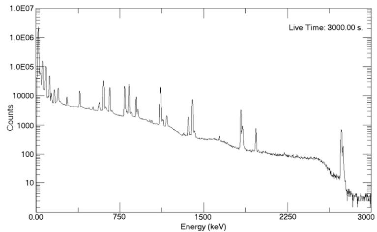
**Figure 3 Calibration Source Spectrum with no Absorber**
