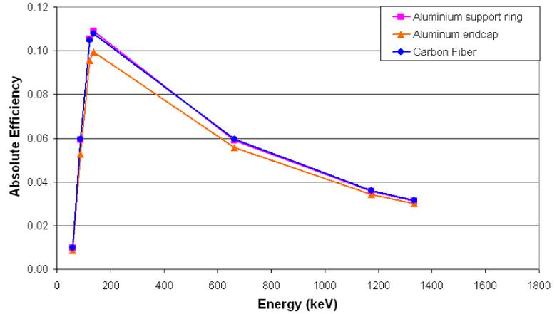
**Figure 4** Comparison of efficiency for different endcaps.
