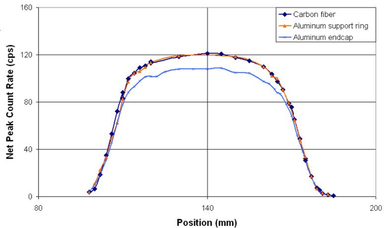
**Figure 5** Comparison of the 59 keV scans of the front face of the detector for different endcaps.
