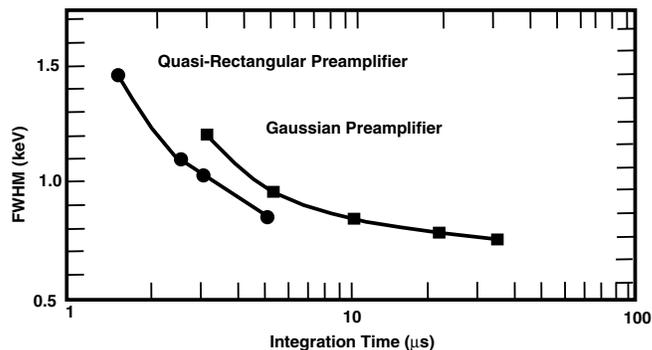
**Figure 7. Noise vs. Integration Time for a Gated Integrator with a Gaussian Prefilter and a Quasi-Rectangular Prefilter.**
