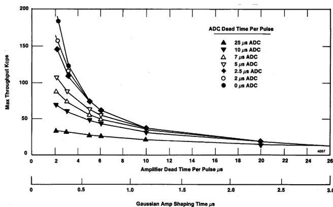
**Figure 6. Maximum Throughput [Calculated, Ignoring TRP Losses, from Equation (1)] for Different ADC Speeds vs. Gaussian Shaping Time.**
