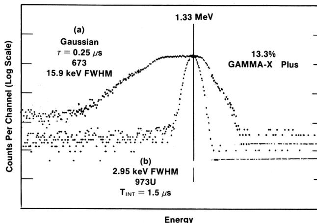
Figure 2. The 1.33-MeV Gamma-Ray Peak from a  $^{60}\text{Co}$  Source, acquired from a germanium detector using (a) an amplifier with a Gaussian pulse shape and a 0.25- $\mu\text{s}$  shaping time constant, and (b) the Model 973U gated integrator amplifier with a 1.5- $\mu\text{s}$  integration time. Vertical scales normalized for peak shape comparison.
