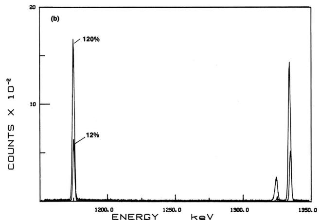
Figure 1B. 1173- and 1332-keV <sup>60</sup>Co Peaks from Figure 1A, Shown on Linear Scale. Peak net areas from the 120% detector are approximately three times as large as those from the 12% detector. (The peak at 1321 keV is a sum peak from <sup>137</sup>Cs in the sample.)
