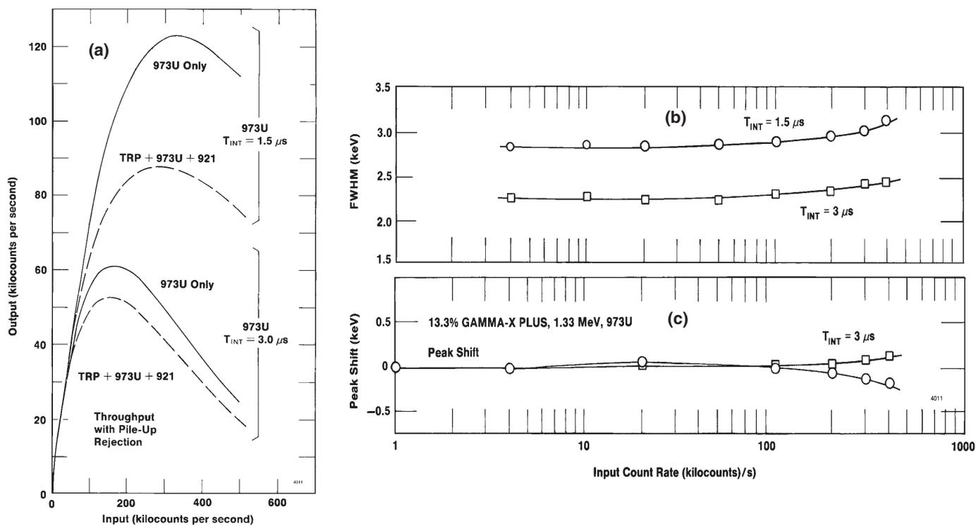
Figure 5. The Throughput-Resolution Trade-Off. (a) Throughput attainable with ORTEC Model 973U gated integrator amplifier at 1.5- $\mu$ s and 3- $\mu$ s integration times; (b) the corresponding resolution curves; and (c) the corresponding stability curves.
