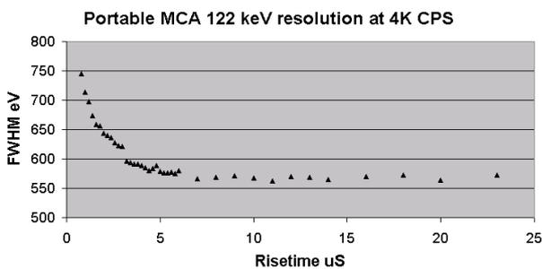
**Figure 4** Portable MCA 122 keV resolution as a function of filter rise time
