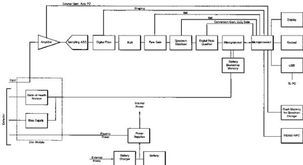
**Figure 1** Portable MCA Schematic Block Diagram
