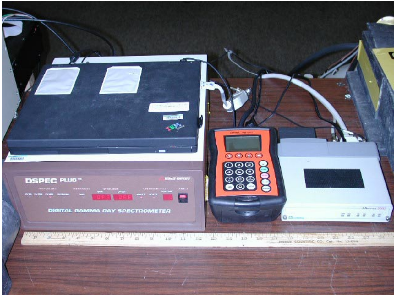
Figure 1: The three DSP systems used in the evaluation. From left to right are the DSPEC Plus, DigiDART, and Inspector 2000. An IBM notebook computer is located on top of the DSPEC Plus.
