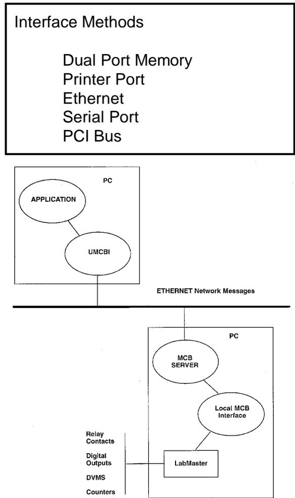
**Figure 9** LabMaster System.
