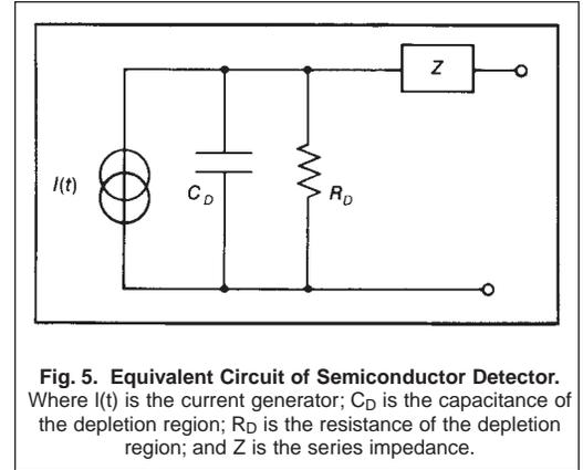
Fig. 5. Equivalent Circuit of Semiconductor Detector. Where  $I(t)$  is the current generator;  $C_D$  is the capacitance of the depletion region;  $R_D$  is the resistance of the depletion region; and  $Z$  is the series impedance.
