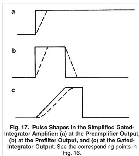
Fig. 17. Pulse Shapes in the Simplified Gated-Integrator Amplifier: (a) at the Preamplifier Output, (b) at the Prefilter Output, and (c) at the Gated-Integrator Output. See the corresponding points in Fig. 16.
