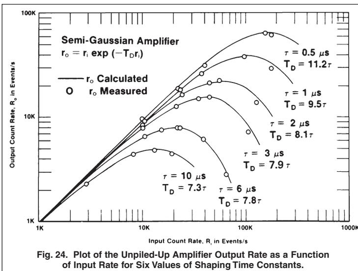
Fig. 24. Plot of the Unpiled-Up Amplifier Output Rate as a Function of Input Rate for Six Values of Shaping Time Constants.
