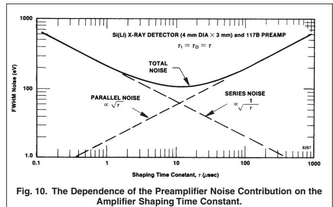
Fig. 10. The Dependence of the Preamplifier Noise Contribution on the Amplifier Shaping Time Constant.
