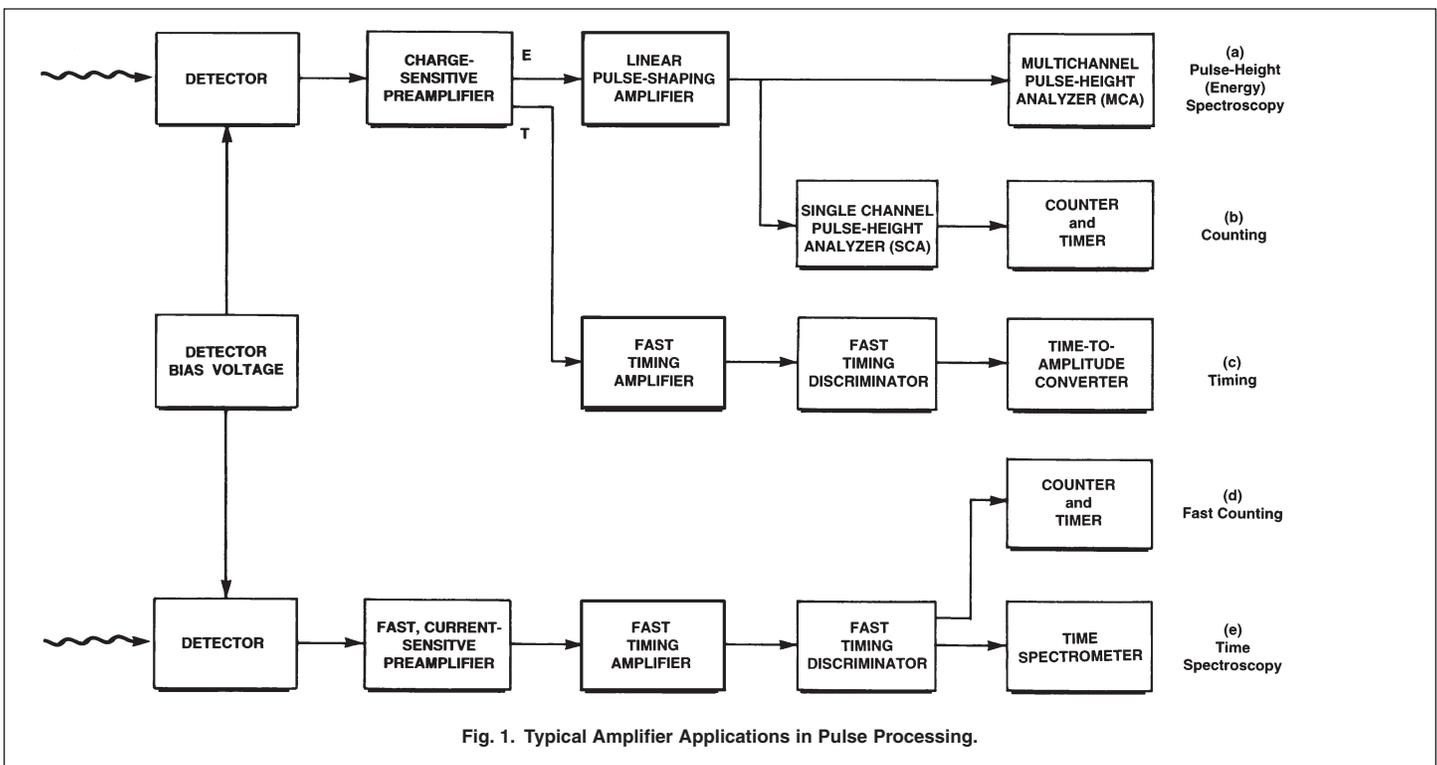
Fig. 1. Typical Amplifier Applications in Pulse Processing.
