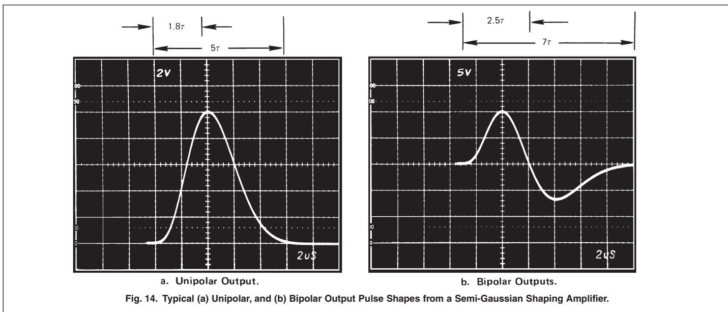
available [Fig. 14(b)]. The bipolar output is useful in minimizing baseline shift with varying counting rates when the electronic circuits following the amplifier are ac-coupled. It is also convenient for zero-crossover timing applications. The drawbacks inherent in the bipolar output relative to the unipolar output are a longer pulse duration and a worse signal-to-noise ratio.
