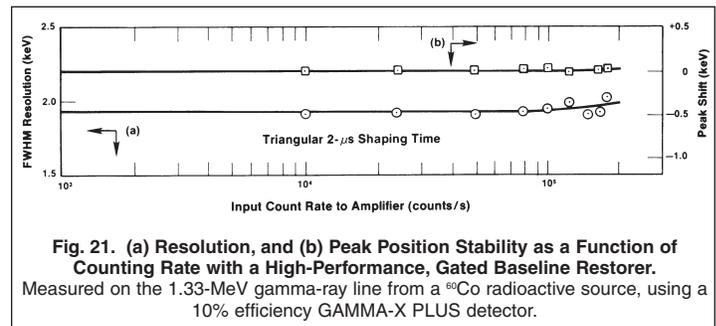
Fig. 21. (a) Resolution, and (b) Peak Position Stability as a Function of Counting Rate with a High-Performance, Gated Baseline Restorer. Measured on the 1.33-MeV gamma-ray line from a  $^{60}\text{Co}$  radioactive source, using a 10% efficiency GAMMA-X PLUS detector.
