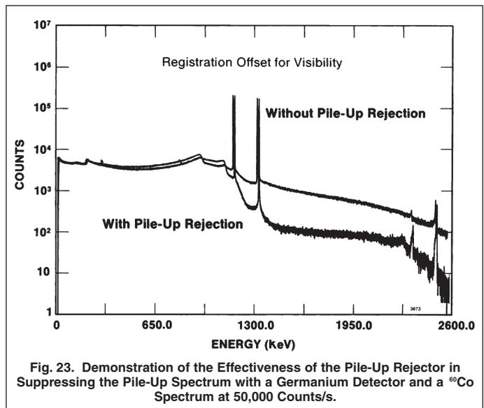
Fig. 23. Demonstration of the Effectiveness of the Pile-Up Rejector in Suppressing the Pile-Up Spectrum with a Germanium Detector and a  $^{60}\text{Co}$  Spectrum at 50,000 Counts/s.
