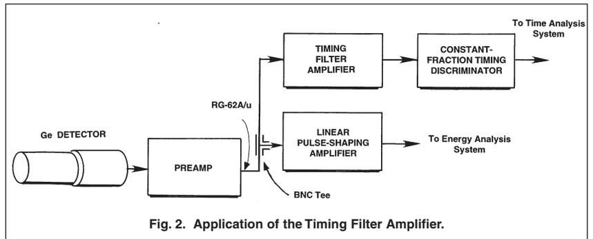
Fig. 2. Application of the Timing Filter Amplifier.
