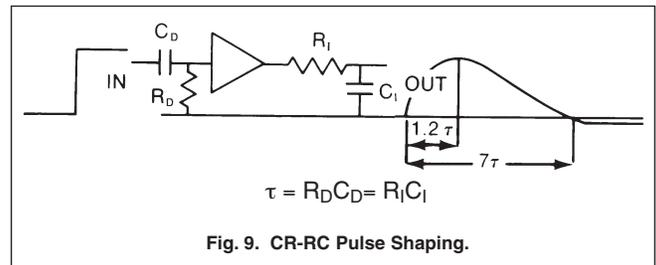
Fig. 9. CR-RC Pulse Shaping.
