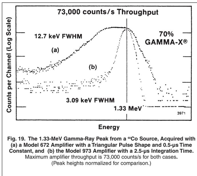
Fig. 19. The 1.33-MeV Gamma-Ray Peak from a <sup>60</sup>Co Source, Acquired with (a) a Model 672 Amplifier with a Triangular Pulse Shape and 0.5- $\mu$ s Time Constant, and (b) the Model 973 Amplifier with a 2.5- $\mu$ s Integration Time. Maximum amplifier throughput is 73,000 counts/s for both cases. (Peak heights normalized for comparison.)
