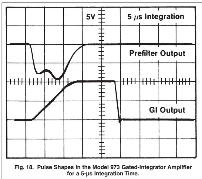
Fig. 18. Pulse Shapes in the Model 973 Gated-Integrator Amplifier for a 5- $\mu$ s Integration Time.
