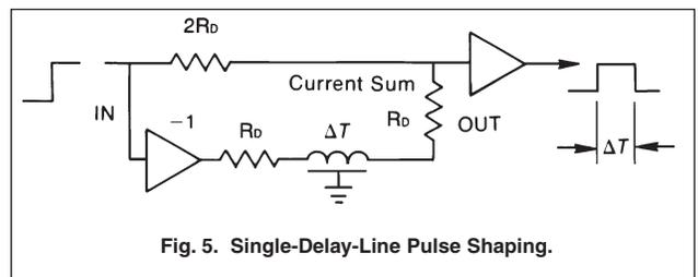
Fig. 5. Single-Delay-Line Pulse Shaping.
