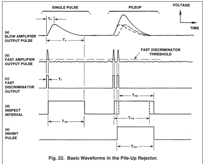
Fig. 22. Basic Waveforms in the Pile-Up Rejector.
