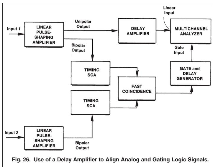
Fig. 26. Use of a Delay Amplifier to Align Analog and Gating Logic Signals.
