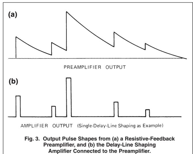
Fig. 3. Output Pulse Shapes from (a) a Resistive-Feedback Preamplifier, and (b) the Delay-Line Shaping Amplifier Connected to the Preamplifier.
