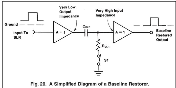
Fig. 20. A Simplified Diagram of a Baseline Restorer.
