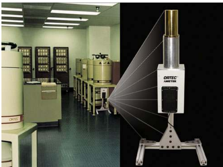
Illustration above showing the LDM100-GEM installed in a standard low background lead shield assembly
