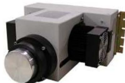
As mentioned earlier, the majority of the gamma-ray emissions from special nuclear material (SNM) are below 1 MeV. Extensive modelling has shown that a detector size of 85 mm diameter by 30 mm deep is an excellent geometry for detecting these gamma rays. The HPGe crystal geometry is nominally the same in all IDMs.
