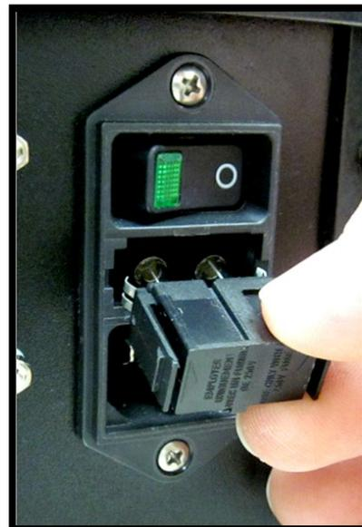
**Figure 8. Inserted Keyed Side Down, Snap Both Sides into Place**
