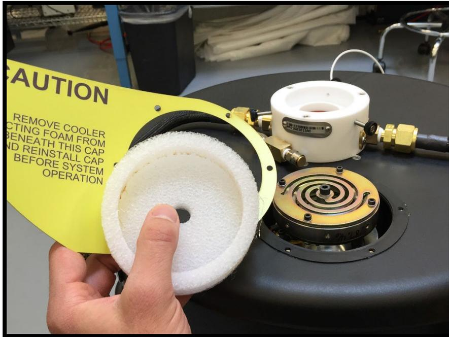
**Figure 6. MÖBIUS with Protective Foam Block and Caution Tag Under Cooler Cover Being Removed**
