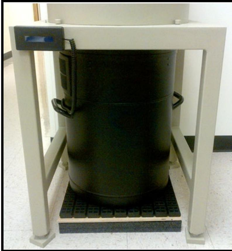
Figure 11. The MÖBIUS Installed on Foam, Plywood, and Anti-Vibration Pad
