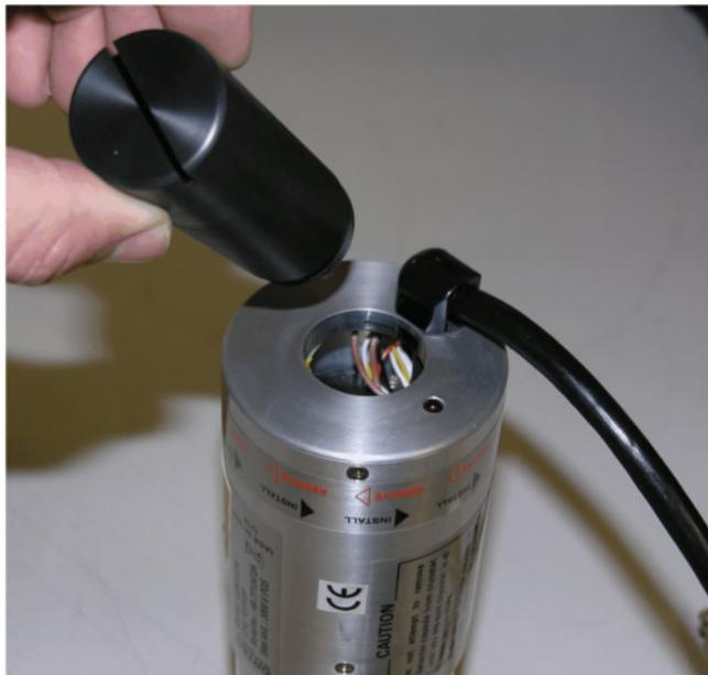
Figure 7. Inserting the shipping plug.
