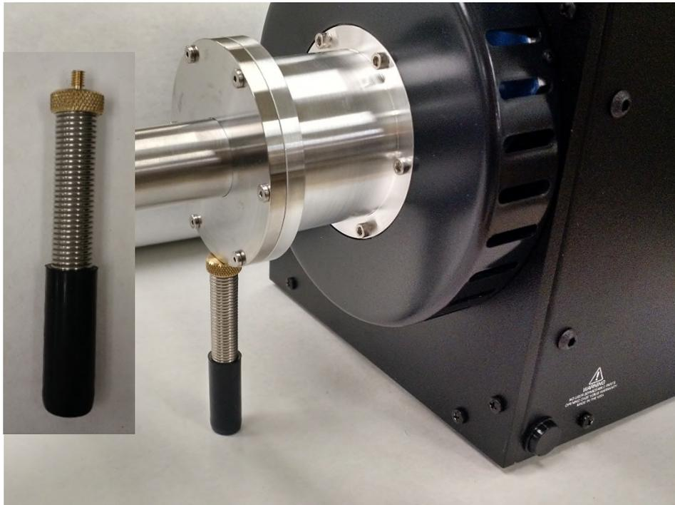
**Figure 6. Horizontal orientation supplemental support installed.**
