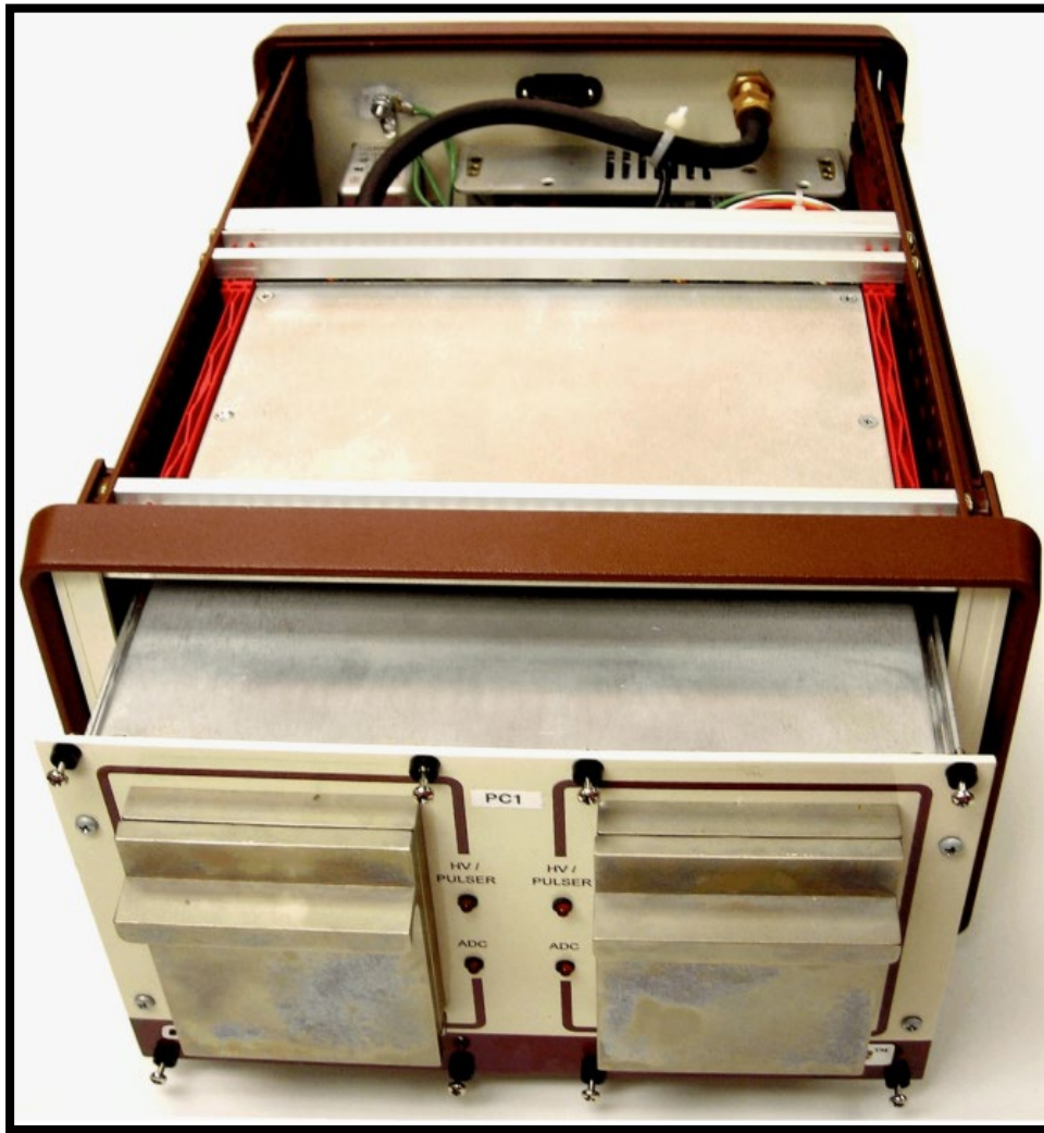
Figure 14. Alpha Duo Partially Removed from Benchtop Enclosure
