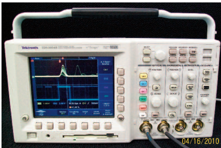
Figure 1.3. The Tektronix Model TDS 3054B Digital Sampling Oscilloscope.
