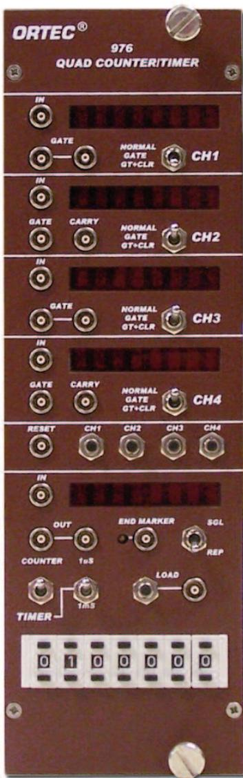
The 976 has four independent 8-digit counters each with their own display and can accept up to 250-MHz input rates. These counters can be cascaded to increase the word length to 16-digits for two counters, and 24-digits for three counters. Counters 2 and 4 have a "Carry" or overflow output to allow the cascading of the counters.
