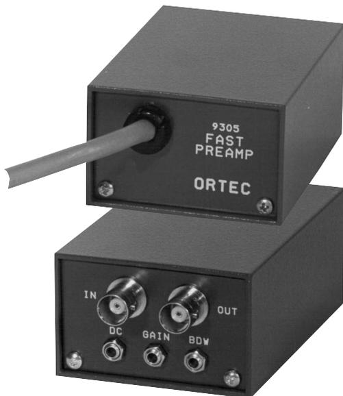
Because of its compact size and light weight, the Model 9305 is ideal for mounting directly on or close to a detector. Consequently, low-level signals which would otherwise be susceptible to distortion by noise or interference are amplified to a suitable level for cable connection to the main amplifier. Connection to a power supply is through a 10-ft cable furnished with the Model 9305.
