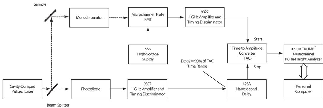
Fig. 1. Typical Block Diagram for a Fluorescence Lifetime Spectrometer (with reversed start/stop assignments).
