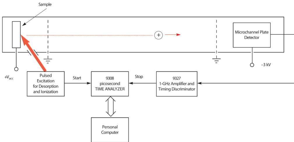
Fig. 2. The Model 9327 in a Simplified Illustration of a Time-of-Flight Mass Spectrometer.
