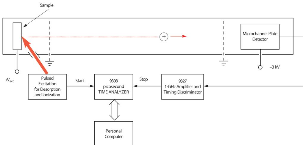
Fig. 2. The Model 9327 in a Simplified Illustration of a Time-of-Flight Mass Spectrometer.
