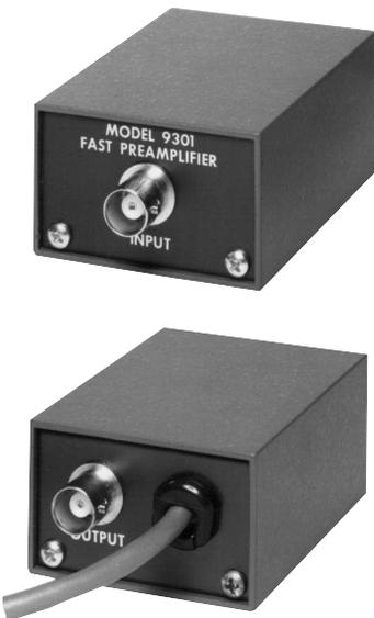
The ORTEC Model 9301 low-noise, fast-rise-time Preamplifier has been designed for use with photomultipliers, electron multipliers, and other detectors employed in photon counting, ion counting, or fast-timing applications. When connected to the detector, the 50- $\Omega$  input resistance of the Model 9301 provides a load resistance for the detector output current pulse.
