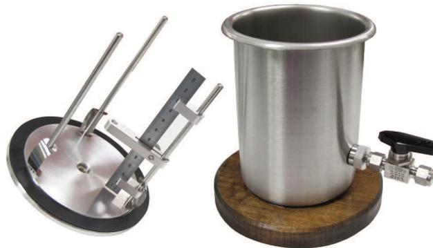
The ORTEC Model 807 Vacuum Chamber is designed for routine alpha/beta counting applications using a semiconductor radiation detector and a radioactive sample. Two examples of the many applications possible with this convenient and durable chamber are its use in educational laboratories to demonstrate detectors and counting principles, and in radiological laboratories for smear counting.
