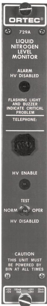
The ORTEC Model 729A Liquid Nitrogen Level Monitor is a single-width module (NIM-standard) designed to serve as an accessory on HPGe coaxial (GEM and GMX), LEPS, Si(Li), and old Ge(Li) detectors in the field.
