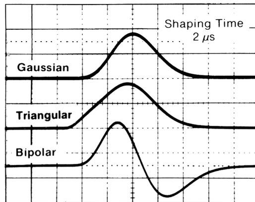
Fig. 1. Gaussian, Triangular, and Bipolar Output Pulse Shapes for a 2- $\mu$ s Shaping Time. Vertical scale, 5 V per division; horizontal scale, 2  $\mu$ s per division.
