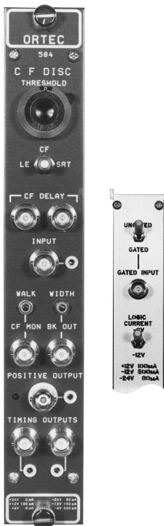
**CF DELAY** Two front-panel BNC connectors accept 50- $\Omega$  coaxial cable to set the required constant-fraction shaping delay for the CF and SRT Modes: total delay is  $\approx 0.8$  ns plus the delay of the external cable. In the LE Mode, the user may either connect a piece of 50- $\Omega$  coaxial cable between these two connectors or connect a 50- $\Omega$  termination to each of the two connectors.
