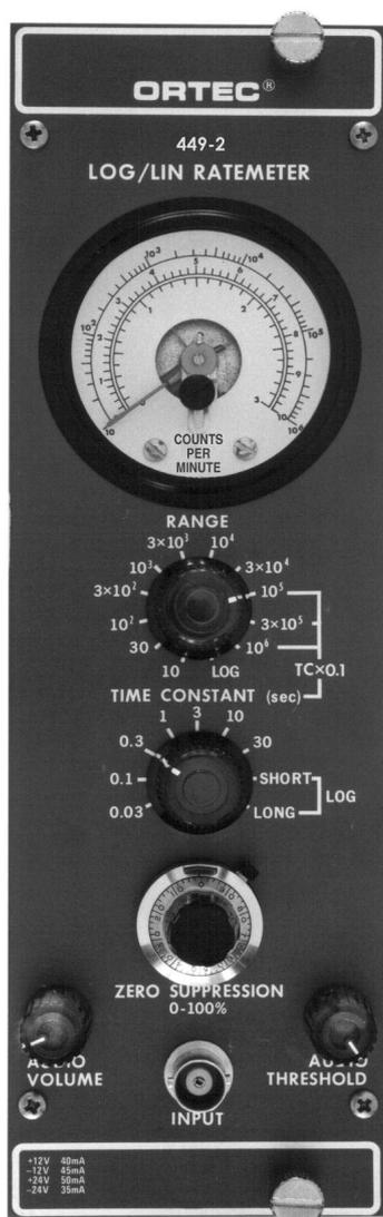
The ORTEC Model 449 Log/Lin Ratemeter provides two modes of operation: linear and logarithmic. The linear mode has 11 full-scale ranges from 10 to 10<sup>6</sup> counts/sec in 1-3-10 steps. The 5-decade log mode covers the range from 10 to 10<sup>6</sup> counts/sec in a single span. These selections permit logical operation of the instrument when measuring low, medium, or high steady pulse rates or when monitoring rates that vary through a wide range.
