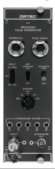
The ORTEC Model 419 is a Precision Pulse Generator that simulates the detection of a nuclear particle reaction in a semiconductor or scintillation detector, as well as serving as a specialized pulse generator for use with pulse processing instrumentation. It can be calibrated to read directly in terms of equivalent energy deposition in semiconductors, and the rise time of the pulse may be varied to simulate the collection time constant in the detector.
