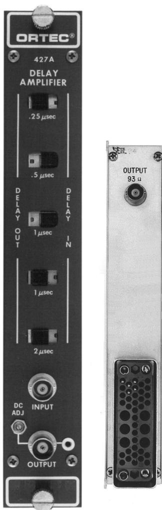
The ORTEC Model 427A Delay Amplifier is suitable for any general-purpose variable delay of linear or logic signals within the range from 0.25 through 4.75  $\mu$ s. All signals, of either polarity and up to 10 V in amplitude, are delayed by the selected time and are reproduced at the outputs. Two outputs are included, one with an impedance nominally 1  $\Omega$  and the other 93  $\Omega$ .
